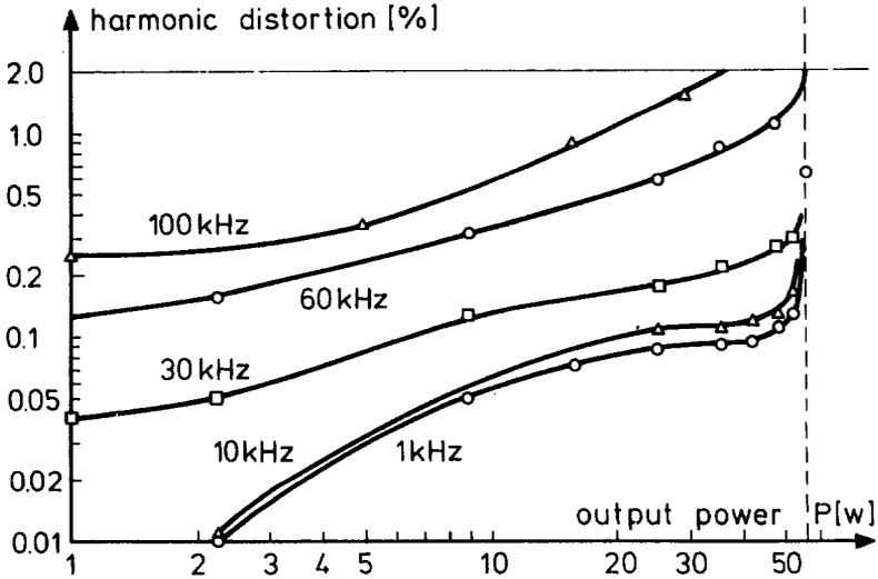
Fig. 5. Total harmonic distortion as a function of power for different frequencies. The distortion at low power levels for frequencies up to 10 kHz is infinitesimally small. No traces of cross-over distortion can be found due to class A operation in the low power range.
