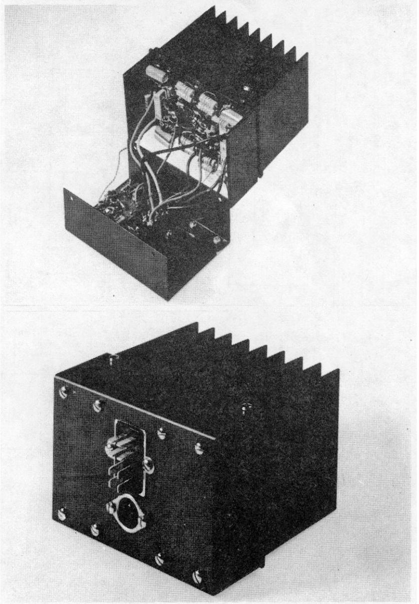
Fig. 2. The mechanical construction of the power amplifier. Transistors T<sub>7</sub>-T<sub>17</sub> are directly mounted on the heat-sink, which has 0.75°C/W thermal resistance to the ambient. The maximum total power dissipation is about 60 W. The input stages are placed on a small printed circuit board which is mounted in the cover. Amplifier dimensions are : 7.5 x 11.7 x 12.0 cm.
