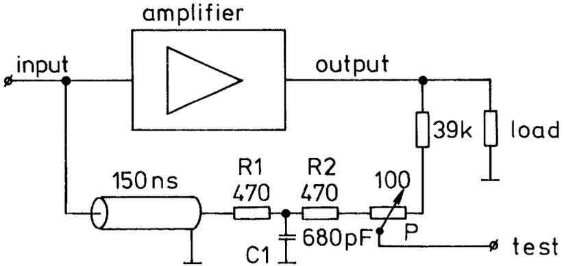
Fig. 8. Compensation test. Because the amplifier is an inverting one, a position can be found of potentiometer  $P$  where the linear component of the output signal exactly compensates the input signal at the "test" point. The momentary discrepancy signal, as scaled up to the output level, was below 0.01% for powers below 5 W and for frequencies in the audio range, and was mainly caused by incomplete phase compensation ( $R_1$ ,  $R_2$  and  $C_1$ ).
