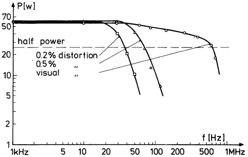
Fig. 4. Equi-distortion curves: power versus frequency for three different criteria. For the proposed criterion of 0.2% total harmonic distortion the amplifier has a power bandwidth of 35 kHz (half power point).
